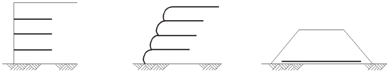
Figure 5.26 Applications in which geogrids are used
