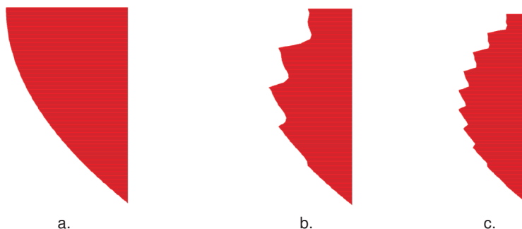
Figure 9.2 Settlement profile of an embankment on a stiff foundation layer: a. Phase displacement results; b. Sum phase displacements results (5 construction layers); c. Sum phase displacements results (10 construction layers)
