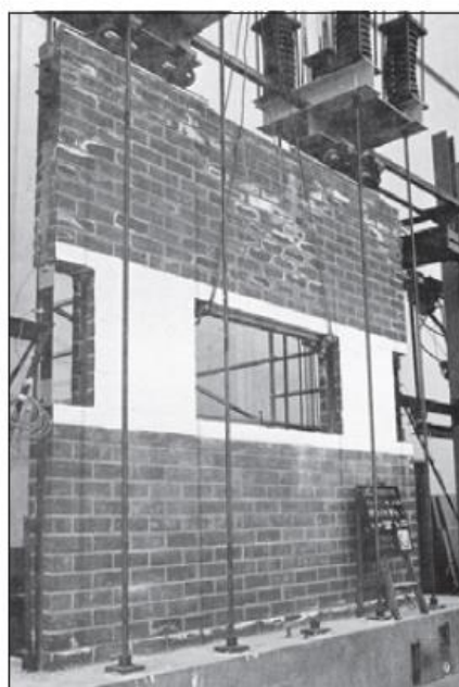
Masonry specimen ready for shake-table testing. Clough headed this mid-1970s project, along with graduate student Ron Mayes. Other graduate students working on the project were Polat Gulkan, Shy Chen, R. Hendrickson, George Manos, and Yutaro Omote.
