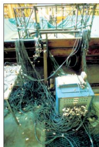
Data acquisition cables for the 1981 water tank shake table testing.
