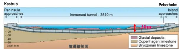
The maximum construction depth is approx. 22 m below water, while the future navigation depth over the tunnel will be dredged to -10 m.
